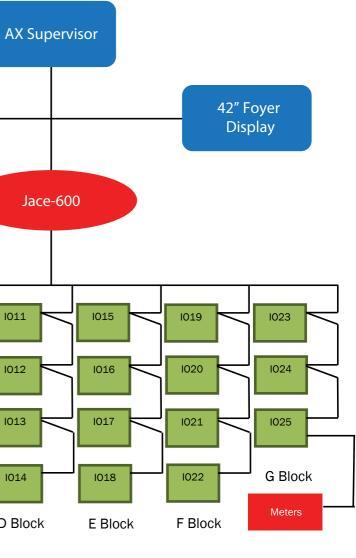
Energy Meters 4 2 x Electrical x Water 2 x Gas Pulsed and RS485
